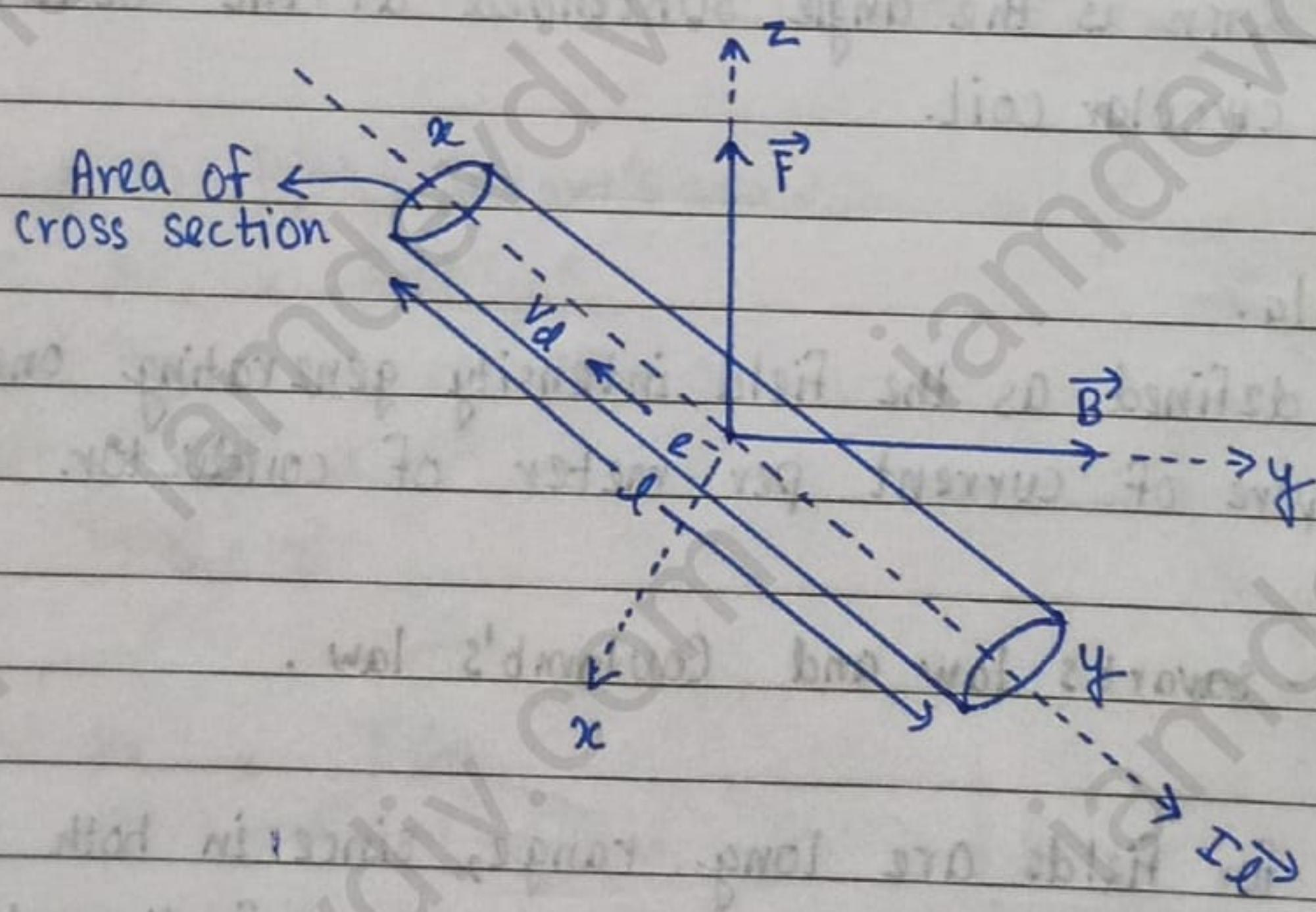
Let's consider a current carrying conductor of length  $l$  is placed in uniform magnetic field  $\vec{B}$
